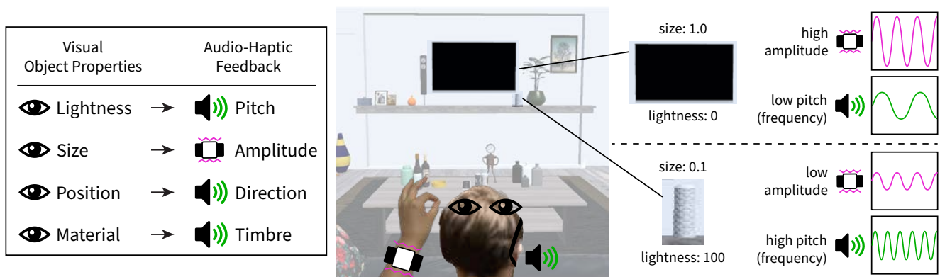
Figure 1: SonoHaptics is an audio-haptic cursor for gaze-based object selection in Extended Reality (XR). SonoHaptics can be activated with a pinch gesture, for example. When activated, it generates unique audio and vibrotactile cues as a user’s gaze hovers over 3D objects, substituting visual feedback. We apply cross-modal correspondence to map visual features of objects to audio-haptic properties. In the visualized scenario, the TV is the largest object in the scene and is black-colored, resulting in high-amplitude haptics on a wristband and low-pitch audio with metal timbre via in-built speakers or earphones. In contrast, the small white vase produces weak vibration and high-pitch audio with ceramic timbre.
