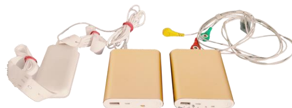
Fig. 2: Two pieces of the Wearable Telecare Multi-Sensor Monitors. On the left, the data acquisition and storage unit with a connected sensor for measuring respiratory activity. On the right, the data acquisition and storage unit with cables for ECG chest electrodes.
