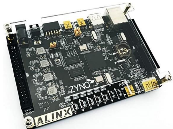
Figure 7. ALINX AX7020: Zynq-7000 SoC XC7Z020 FPGA Development Board
