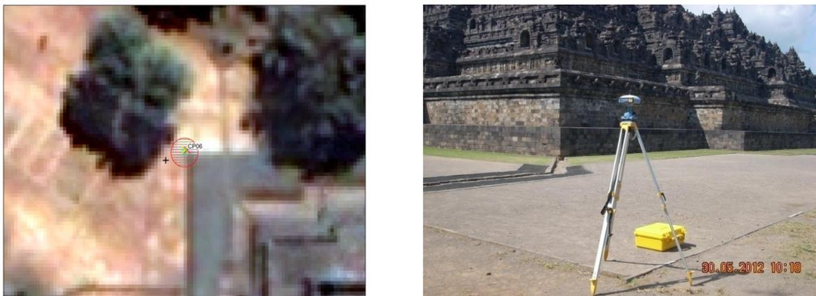
**Figure 1.** GCP measurement with GNSS and its identification on VHRS imagery.
