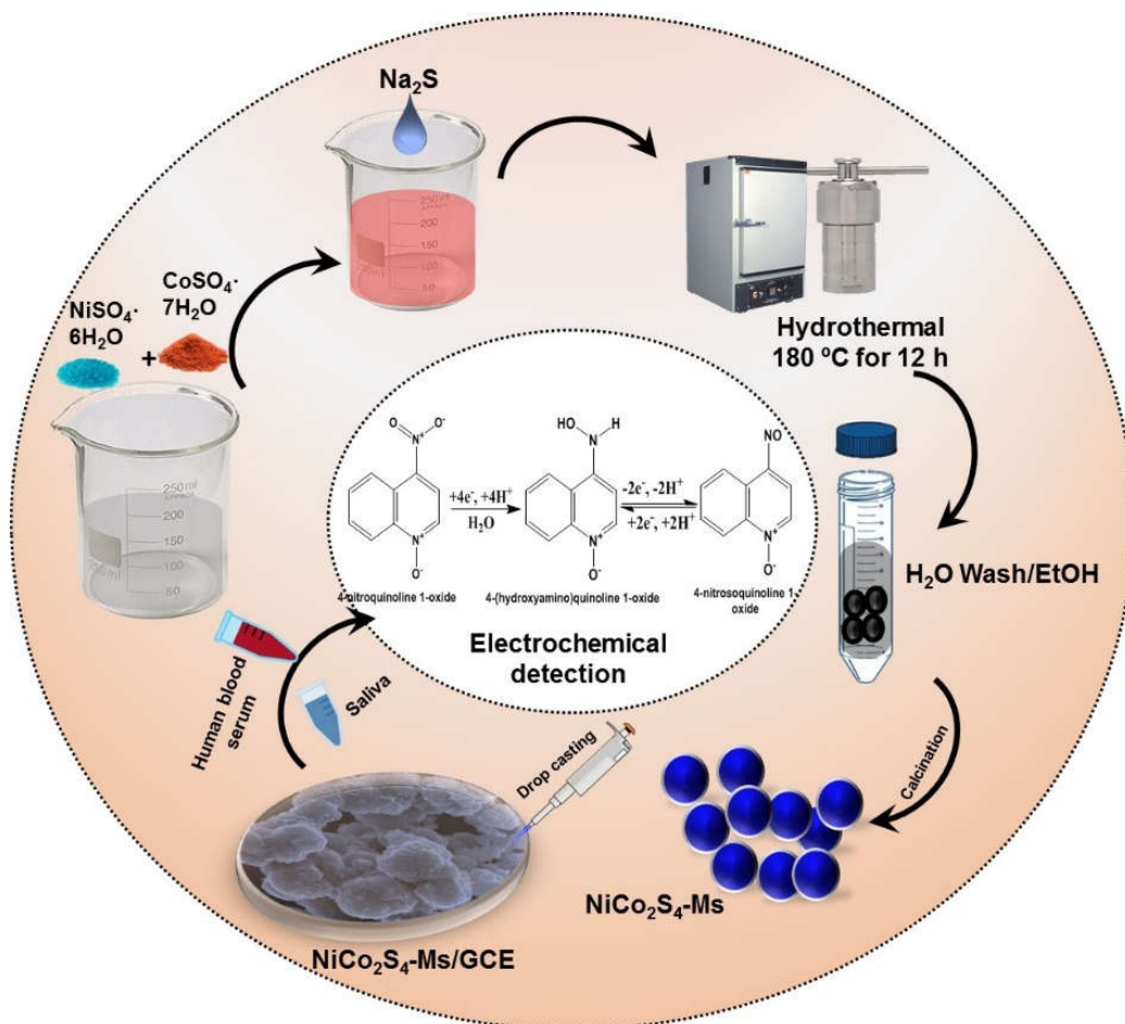
Scheme 1. Synthesis methodology of NiCo 2 S 4 -Ms and its electrocatalytic properties for the detection of 4-nitroquinoline n-oxide.
