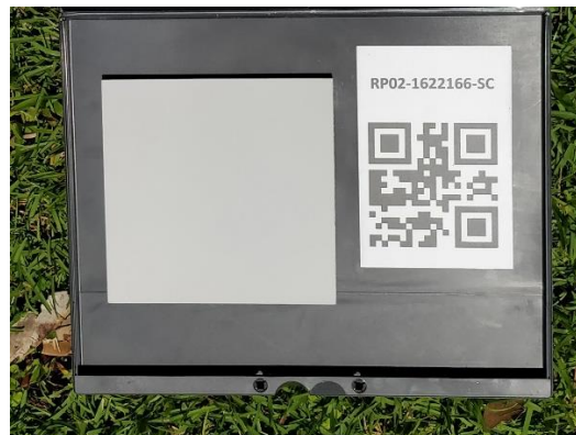
Figure 1. Image of the calibrated reflectance panel, which was captured before each flight. Using the calibrated reflectance panel enabled more accurate compensation for incident light conditions and generation of quantitative data.
