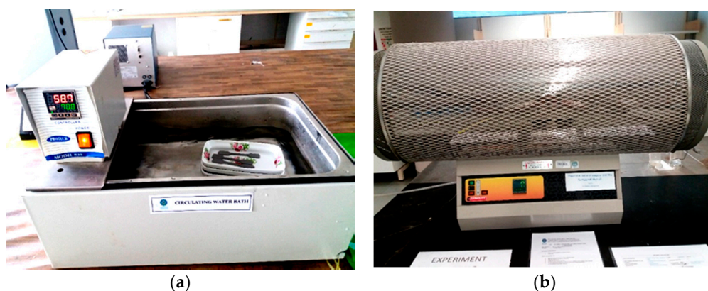
Figure 5. (a) Solvent de-binding of MIM green parts and (b) furnace for thermal de-binding and sintering of MIM brown parts.
