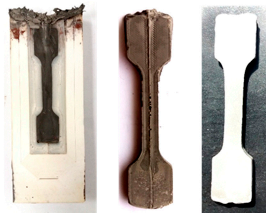
Figure 11. Nylon split mold with green and sintered MIM parts.
