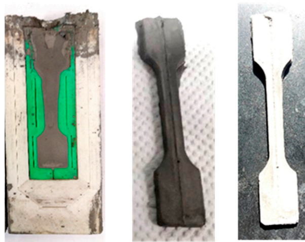
Figure 10. ABS split mold with green and sintered MIM parts.
