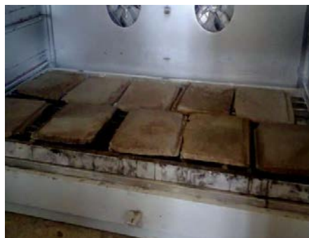
Fig. 6. Specimens in hot air oven for dry (or temperature) curing
