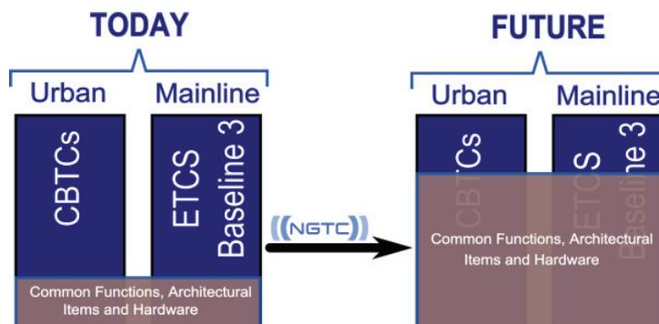
Fig. 1. Expected specifications convergence thanks to NGTC project.
