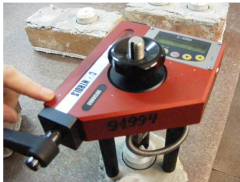
Fig. 1. CONTROLS 58-C0215/T Pull-Off tester.
