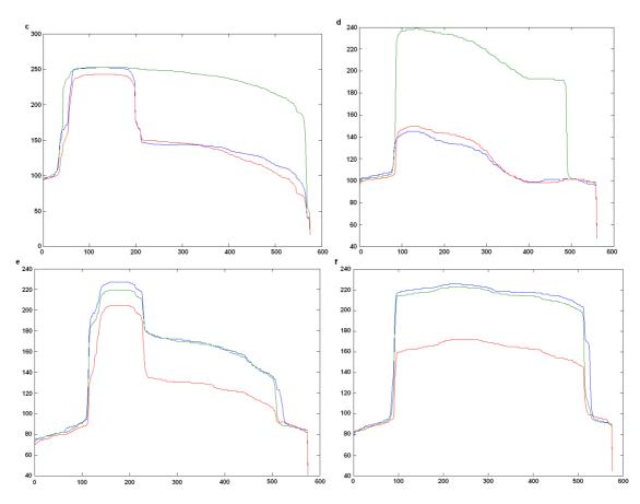
Figure 5. The wave forms of three primary colours of different bobbins. (a) The portion with yarn on purple bobbin. (b) The portion without yarn on purple bobbin. (c) The portion with yarn on green bobbin. (d) The portion without yarn on green bobbin. (e) The portion with yarn on yellow bobbin. (f) The portion without yarn on yellow bobbin
