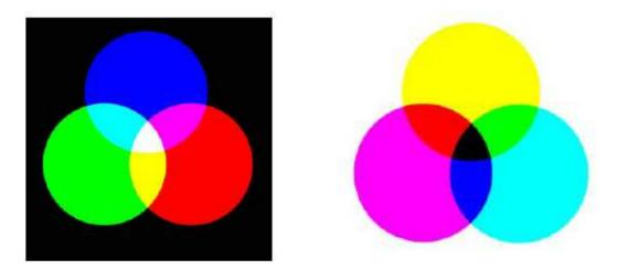
Figure 1. Diagram of trichromatic principle
