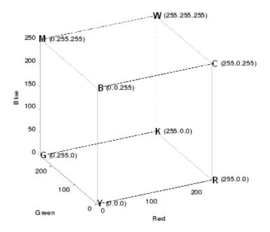
Figure 2. Three orthogonal axes represent R,G and B respectively. The maximum of these three variables is 255. The eight apexes represent red (R), green (G), blue (B), purple (C), cyan (M), yellow (Y), white (W) and black (K) in printing color.
