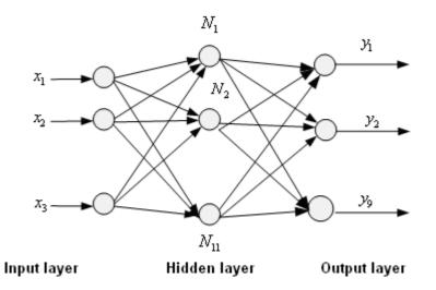
Figure 3. The model diagram of BP neural network based color recognition
