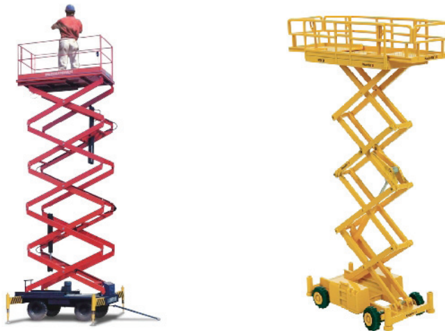
Fig. 3. (a) two hydraulic cylinders driving type platform; (b) one hydraulic cylinder driving type platform
