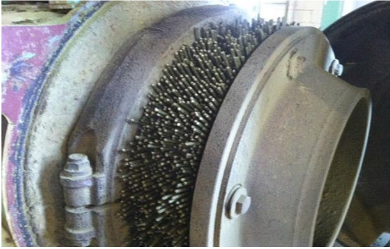
Fig. 1. Industrial pellet mill for biomass pelleting (Dien et al., 2018)
