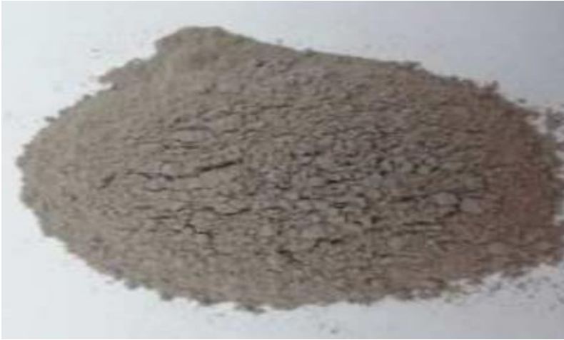
Fig. 3. Bone meal crushed for 75 \mu\text{m} (200 mesh) (Payus et al., 2014)
