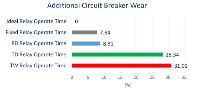
Fig. 13 Additional circuit breaker wear comparison
