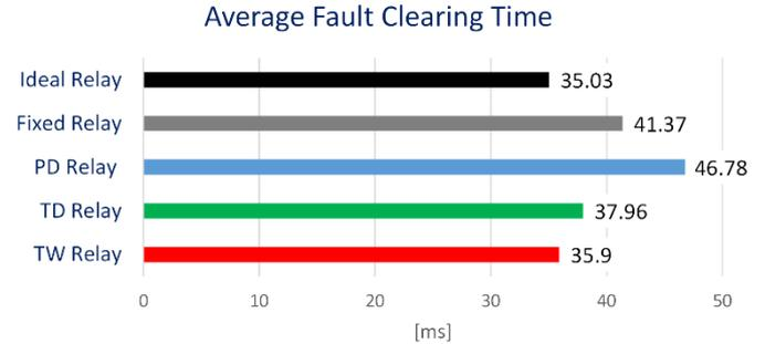
Fig. 12 Average fault clearing time comparison
