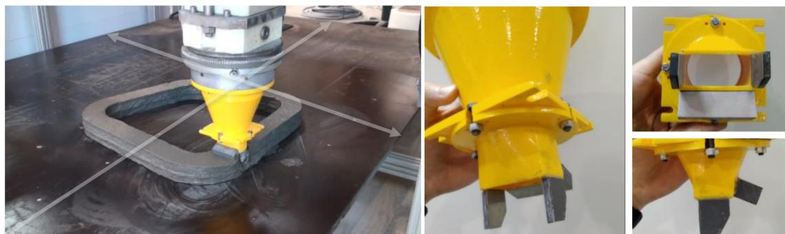
Figure 2: Picture of the nozzle and a printed module (left); Detailed picture of the nozzle with side and back trowels
