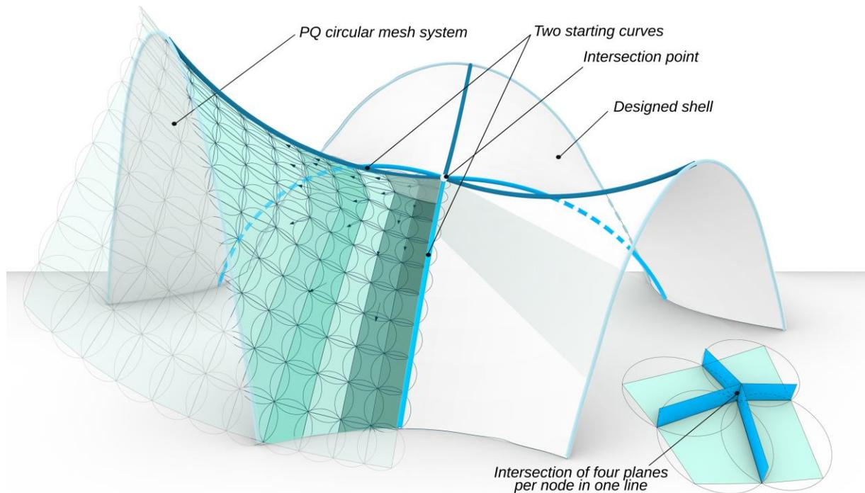
Figure 6: PQ circular mesh generation from two curves on one part of the free form shell design with detail explaining no geometry torsion solution for prefabrication
