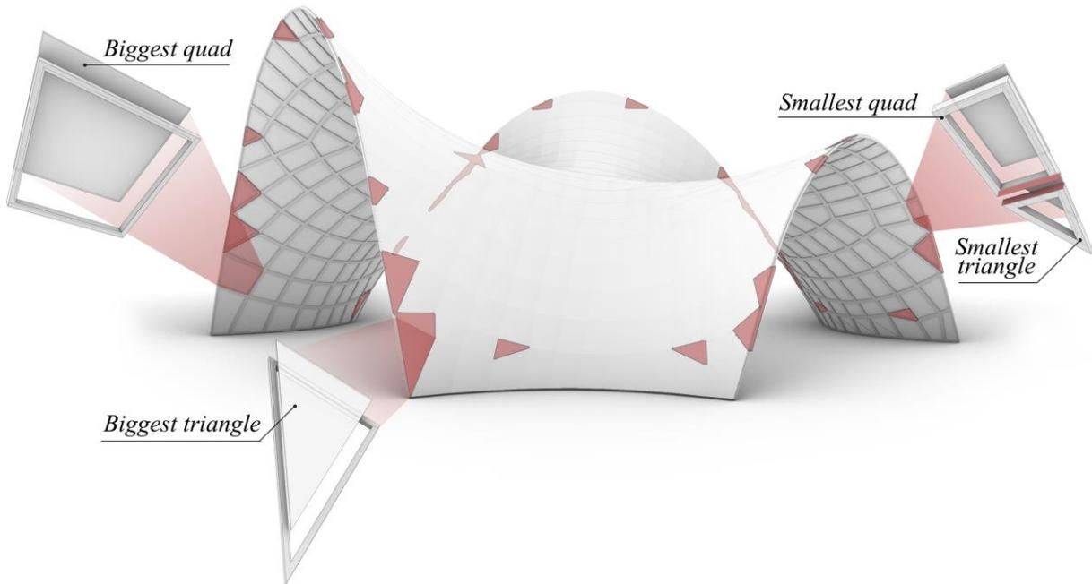
Figure 9: The final shell presented with four characteristic and highlighted triangle modules
