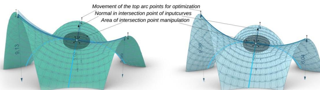
Figure 7: Display of the two solutions from the Galapagos optimization process with input parameters
