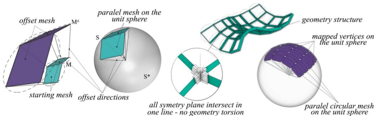
Figure 5: Mesh offset properties of the circular mesh system within the unit sphere (left) and computed for the entire structure (right)
