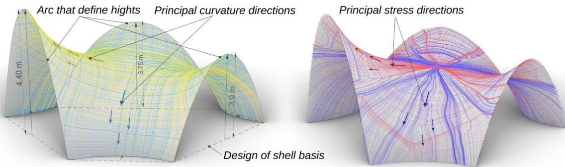
Figure 4: Starting free form shell design with analyzed principal curvature and stress directions
