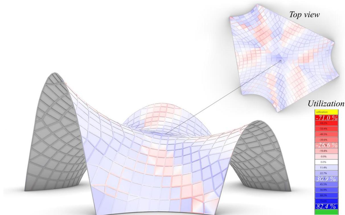
Figure 8: Display of the shells calculated utilization in perspective and top view with critical numbers in the scale
