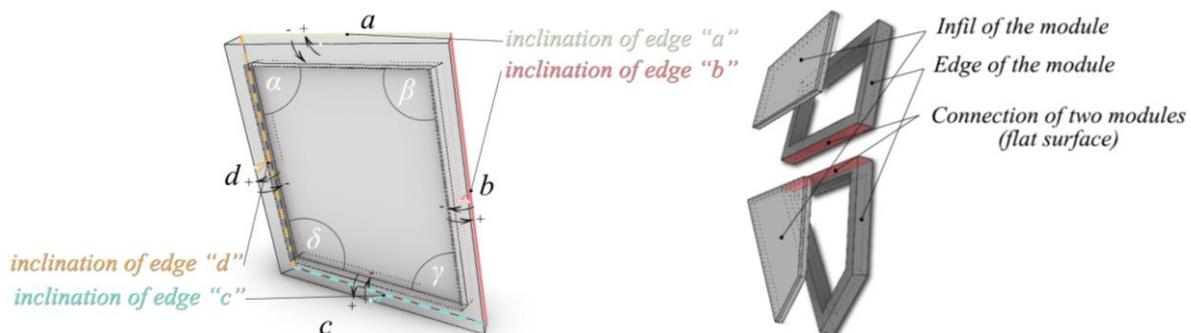
Figure 1: Representation of the module as a unit for 3D concrete printing in free-form shell construction with its distinguished parts
