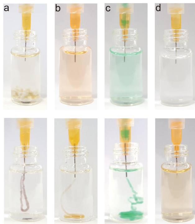
Fig. 8 Macroscopic images of the pre-molding mixture following extrusion into Tris-HCl buffer (pH: 3.5 up, pH: 8.0 down). Pre-molding Fe 3+ -induced HA-Cat gel solution mixture (a), pre-molding NaIO 4 -induced HA-Cat gel solution mixture (b), pre-molding HA-Cat & HA-SH gel solution mixture (c), pre-molding HA-Cat & HA-NH 2 gel solution mixture (d).
