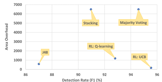
Fig. 5: Detection rate vs. area overhead comparison of RL (UCB, Q-learning), ensemble (majority voting, stacking) and best ML model (J48).
