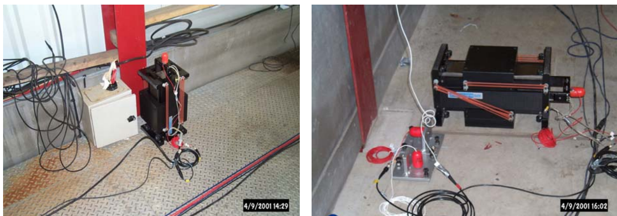
Figure 4: APS Dynamic Model 113 Shaker in (a) vertical and (b) horizontal directions
