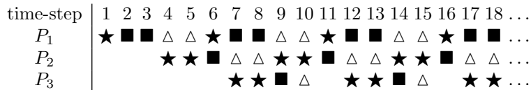
FIGURE 8.14: An example of one-to-one mapping with three stages and processors. Each processor periodically receives input data from its predecessor (★), performs some computation (■), and outputs data to its successor (△). Note that these operations are shifted in time from one processor to another. The cycle-time of P_1 and P_2 is 5 while that of P_3 is 4, hence T_{\text{period}} = 5 .
