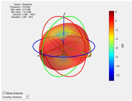
**Fig. 5:** 3 Dimensional radiation pattern of the proposed antenna augmented on the antenna design
