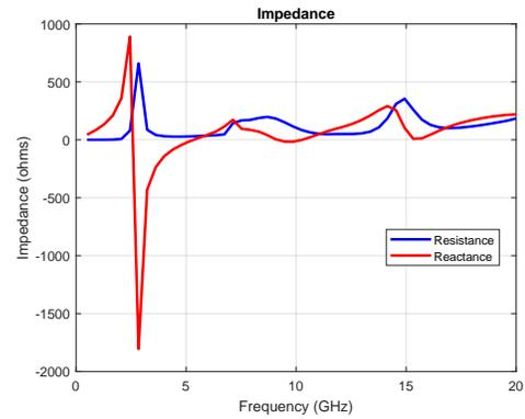
**Fig. 4:** Impedance of the proposed antenna.
