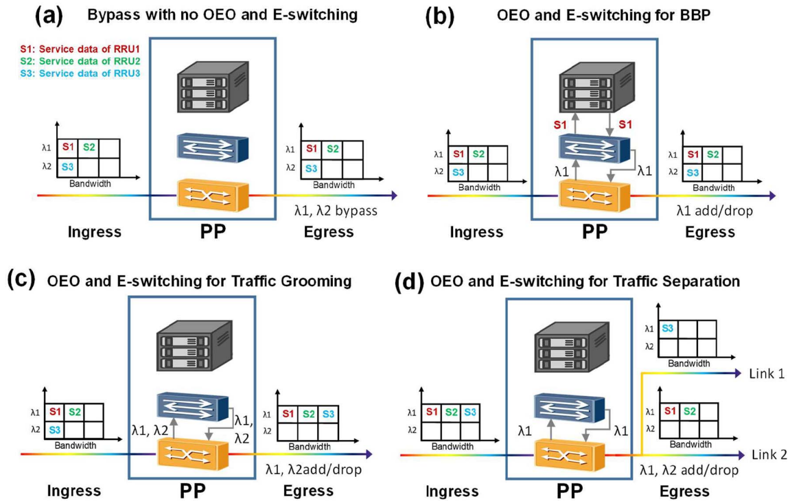
Fig. 4. The OEO conversion and E-switching operation for (a) bypass; (b) baseband processing; (c) traffic grooming; (d) traffic separation.
