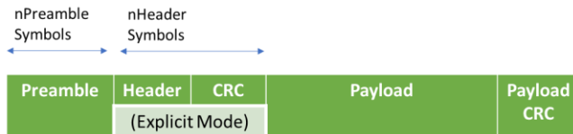
Figure 8. LoRaWAN packet formatting
