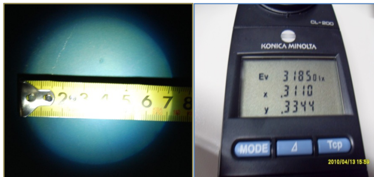
Fig. 5. The spot size and the illuminance of the headlight made of 5 W LED.
