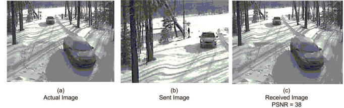
Fig. 13. (a) Actual image from WDW dataset (b) The upper left portion of the image in (a) is sent to the sink node (c) The reconstructed image after superimposing the received image on the stored image for a particular sensor node
