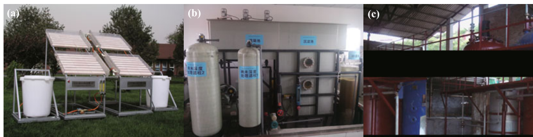
Fig. 19 (a) A trial unit for degrading organic pollutant by sun light; (b) A trial unit to remove arsenate in drink water using combined flocculation and adsorption technique; and (c) A trial unit to remove Cr (VI) from industrial waste by phase transformation.
