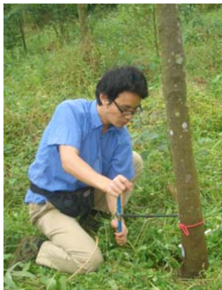
Figure 2. Wood core sample extraction from a 6-year old sandal at 30cm above ground level using an increment borer.
