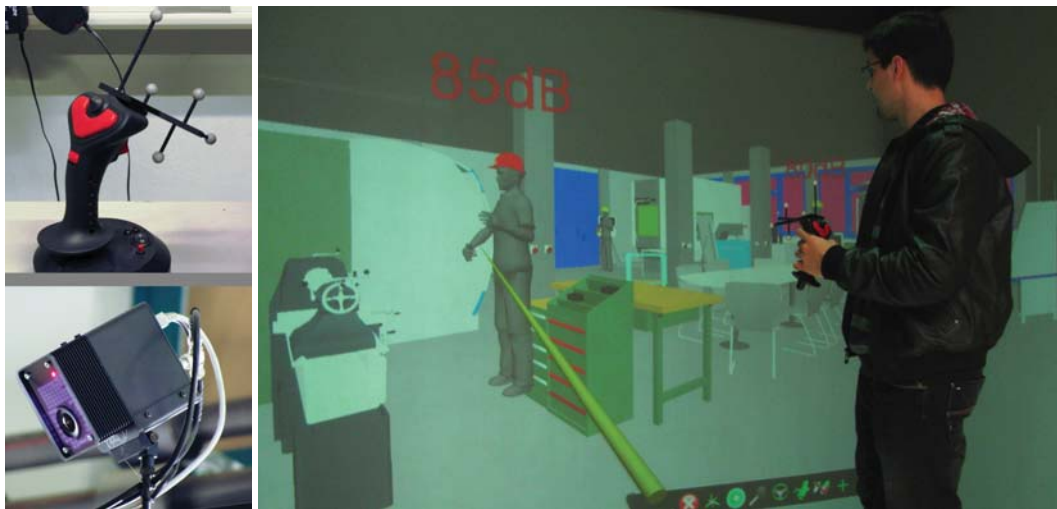
(a) IR tracking system (b) Sound pressure level visualization in CAVE
