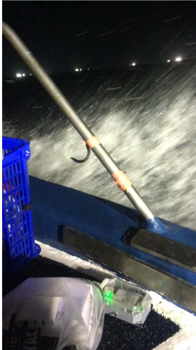
Figure 9: Testing i-Fish. The device is placed at the bow of the vessel close to the starboard side. The waves can crash onto the fishing vessel and soak the device.
