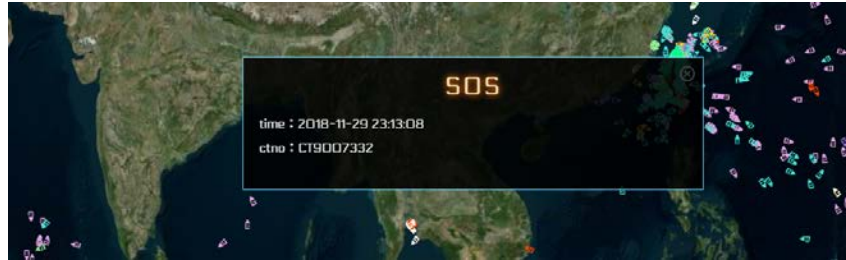
Figure 11: Emergency alert. By pressing the emergency button on the i-Fish device, the central monitoring system will show a big notification showing information of the vessel that sent the distress call.
