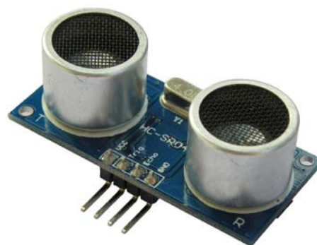
Fig. 2. The HC-SR04 ultrasonic distance sensor.
