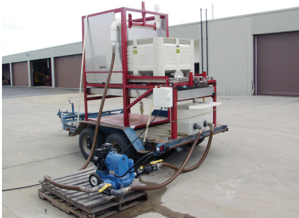
Figure 1 Portable automated bin drencher developed for testing various decay control treatments applied to apples and pears before storage. A small reservoir tank allows for testing small volumes on an entire bin. This is particularly important with biocontrol agents, where limited amounts are available because they are often grown in small fermenters under laboratory conditions (Janisiewicz and Peterson, 2005).
