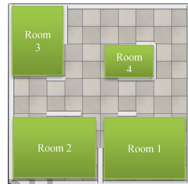
Figure 1. Continuous map on V-Rep simulator. Green areas represent the rooms while the rest is corridor.
