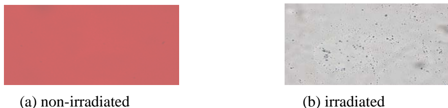
Figure 2 Photographs of LR-115 with neutron from Am(Be) source (40x)
