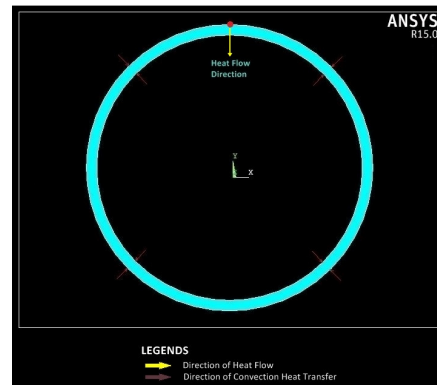
Fig. 6 Developed ANSYS 2D finite element model (without fluid introduction)
