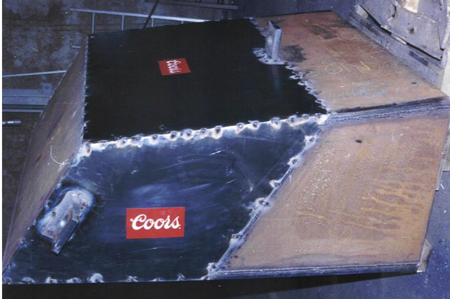
ARL ceramic/glass composite target
