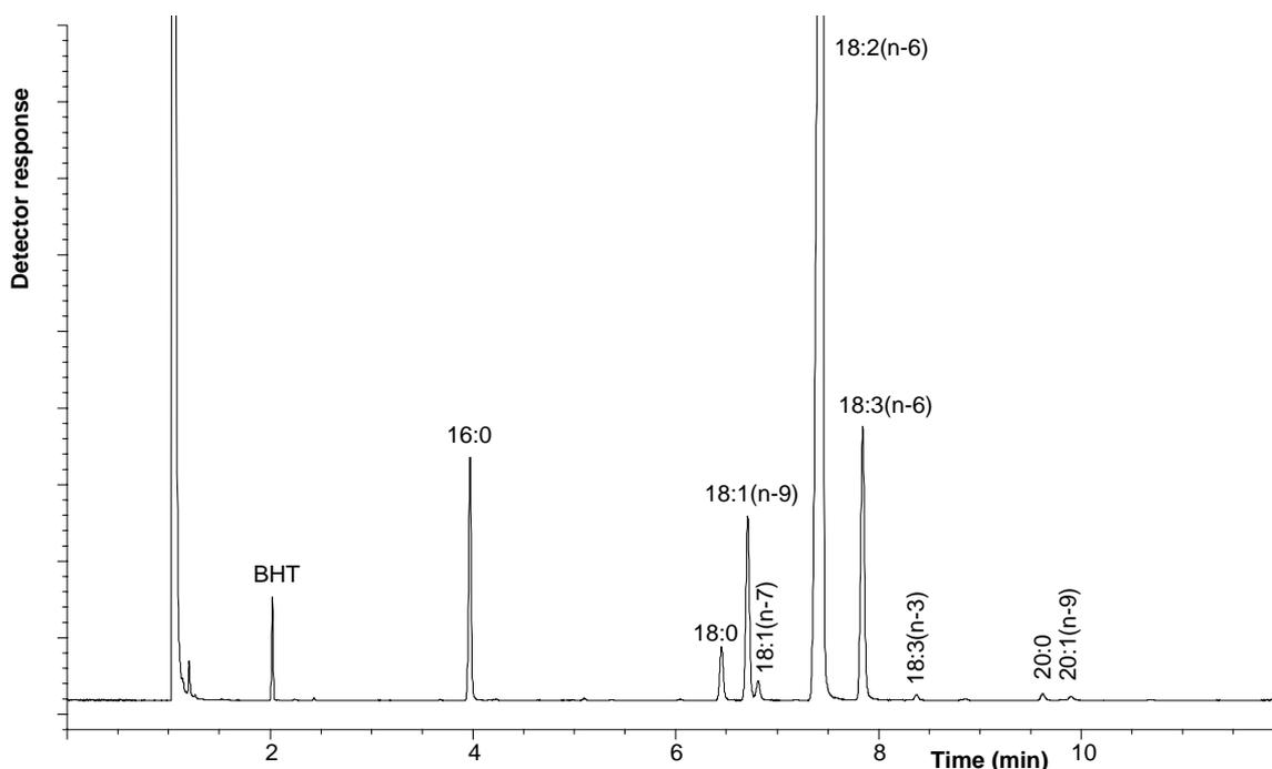
Fig. 1. GC separation of methyl esters of fatty acids from evening primrose oil. A Hewlett Packard Model 5890 Series II gas chromatograph (Hewlett-Packard Ltd., Stockport, Cheshire, U.K.) with a split/splitless injection system, was equipped with a capillary column (25 m x 0.22 mm i.d.) of fused silica coated with Carbowax 20M. The initial temperature of 170°C was held for 3 min and then programmed up to 210°C at 4°C/min, with a final hold for 10 min. Hydrogen was the carrier gas.
