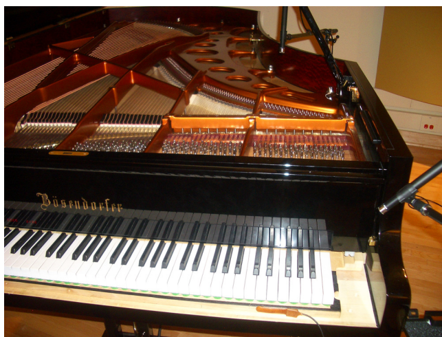
FIG. 5. (Color online) The stimuli were played and recorded on this Bösendorfer CEUS computer-monitored grand piano. The stimuli for the experiments were taken from the microphone to the right of the keyboard. The contact microphone and the microphone further back pointing toward the piano strings are not used in this experiment.
