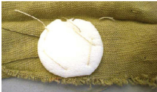
Figure 4. The isolation of the sensor inside the belt.
