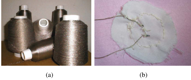
Figure 6. (a) Conductive textile yarn and (b) the connections of the conductive textile wires and the NTC sensor.
