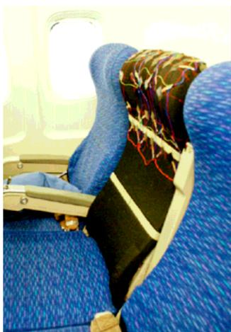
Fig. 3. FSR sensors on head rest area
