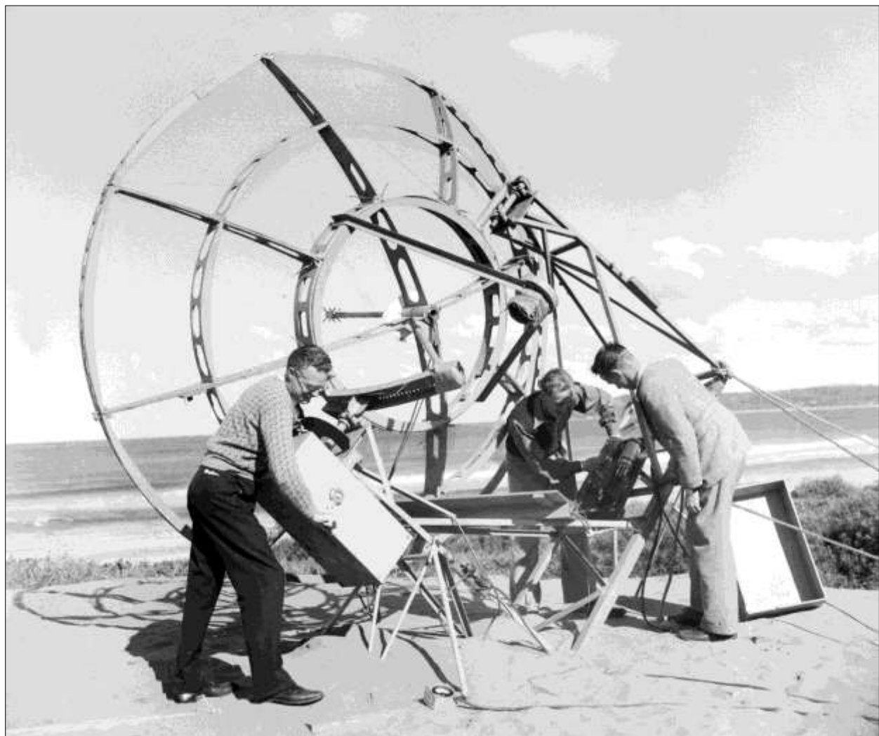
Figure 11: An AN/TPS-3 aerial being set up at Eaglehawk Neck in Tasmania for the 1949 eclipse observations. From left to right are Jack Harragon, John Murray and Don Yabsley (courtesy: The Mercury newspaper).
