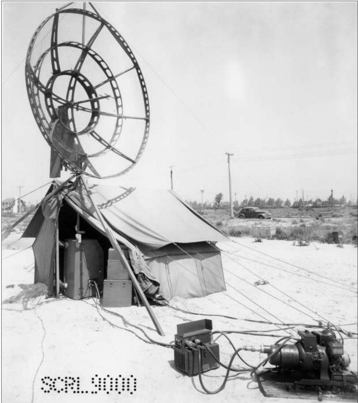
Figure 3: The AN/TPS-3 Radar at Camp Evans, Belmar, New Jersey (USA) on 16 June 1944. In the foreground is the single cylinder gasoline engine used to drive a 400 Hz alternator and a DC generator mounted on the same shaft. Inside the tent are the transmitting and receiving equipment (courtesy: CE LCMS Historical Office Department of the Army, USA).
