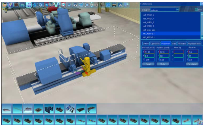
Fig. 5. Example of roll shop reconfiguration: addition of a roll grinder. The icons of the resource catalog can be noticed at the bottom of the screenshot. The user interface in top-right corner provides details about the selected object.
