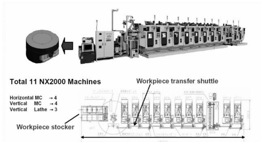
**Fig. 3.5** Impact of small machines at a system level – Travel distance is reduced by 30% compared to previous models (Courtesy of Mori Seiki)
