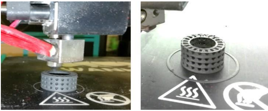
Fig. 1: FFF printed part on the printing bed, left: hard metal, right: cermet
