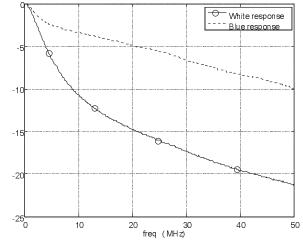
Figure 2. Small-signal modulation bandwidth of LUXEON STAR device
