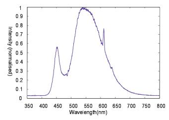
Figure 1. Emission spectrum from white-light LED (LUXEON STAR)
