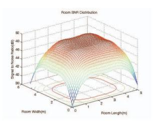
Figure 4. Signal to noise ratio as a function of receiver position
