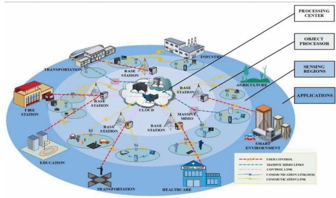
Fig. 2. The architecture of the 5G I-IoT
