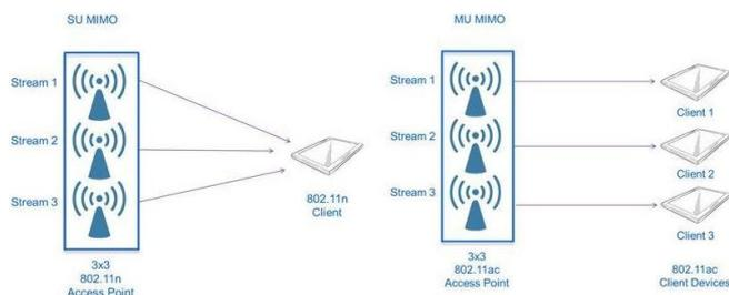
Fig. 3. Differences between SU-MIMO and MU-MIMO Source Adapted from [34]
