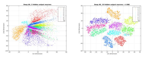
Fig. 5. Visualization of MNIST test set in a 2D space by 2D (left) and 10D (right) deep AE
