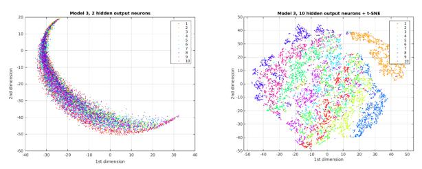
Fig. 8. Visualization of MNIST test set in a 2D space by 2D (left) and 10D (right) Model 3
