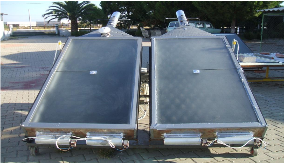
Figure 1. Experimental setup of the solar air collectors (Flat Type on the left and Conic Type on the right)
