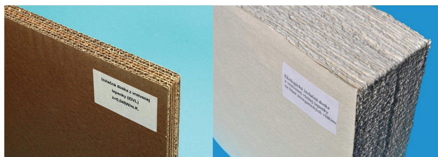
Fig. 2: Thermal insulation boards based on an old corrugated carton.
