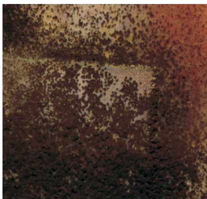
Figure 6. Aspergillus niger and Aspergillus flavus moulds spontaneously grown on the wet-white leather sample tanned with resorcinol-oxazolidine after 21 days
