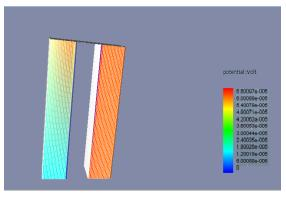
Fig 7 Potential distribution of thermocouple obtained in Thermo electric module in intellisuit software.
