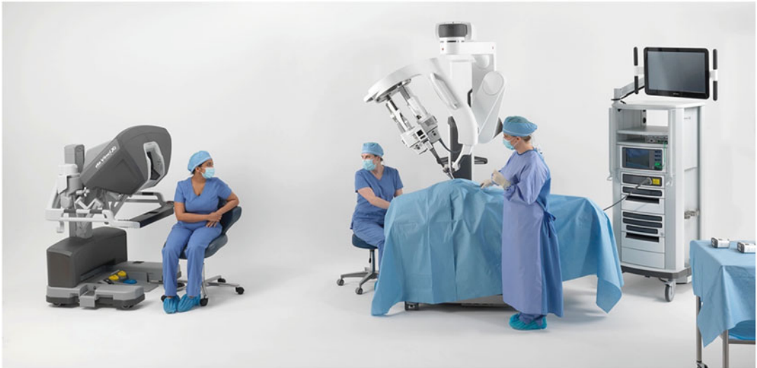
Fig. 59.5 The da Vinci® Surgical System has three main integrated subsystems: (L–R) the surgeon console, patient cart, and the vision cart (with permissions from Intuitive Surgical, Inc.)
